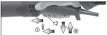
**Switching on:** Switch the machine on as described above. Now slide the trigger switch (12) forwards again and release in the front position to lock the trigger switch (12) (continuous operation).
