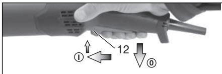
**Switching on:** Slide the trigger switch (12) forwards and then push the trigger switch (12) upwards.
